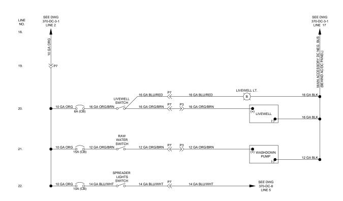
12V DC Cockpit Switch Panel Diagram
