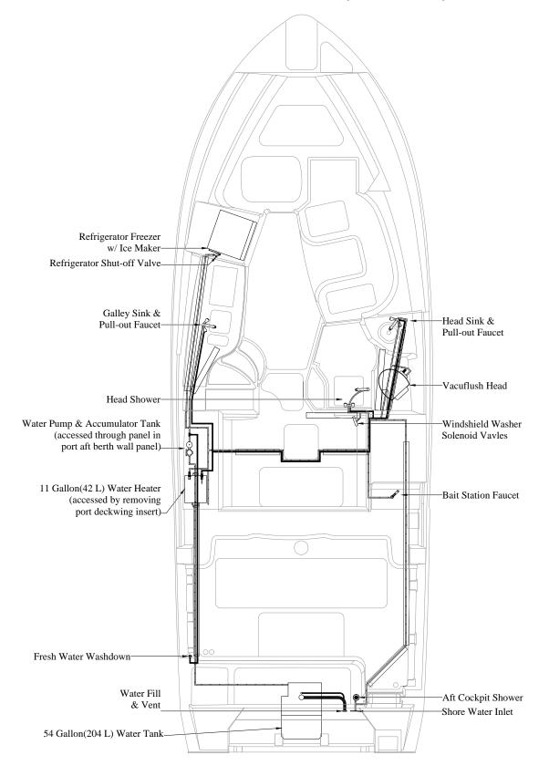
Pressurized Freshwater System Layout
