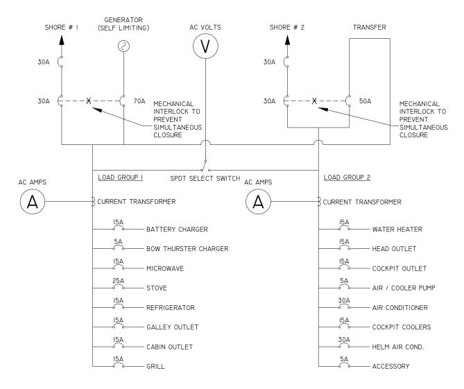
NOTE: WHEN OPERATING FROM A SINGLE POWER SOURCE WITH THE TRANSFER SWITCH ENGAGED, THE AMP READINGS MUST BE ADDED FOR PROPER LOAD MANAGEMENT.
