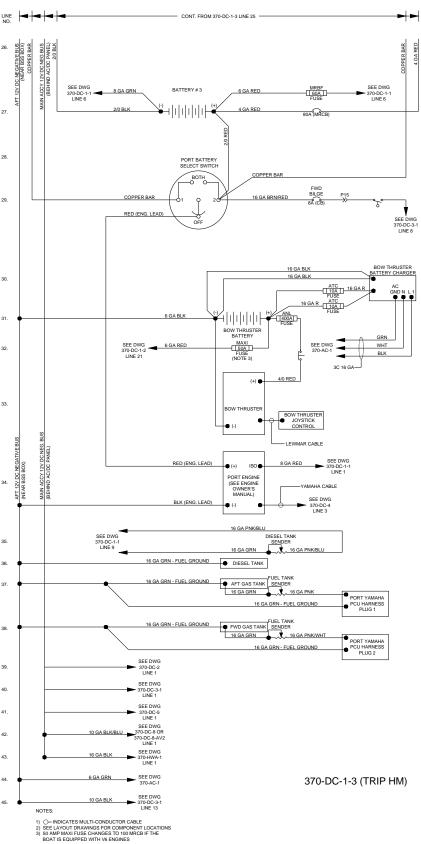
12 Volt DC Electrical Diagram - Triple Engines with Power Assist Option
